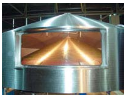
A window into a Merlin wort-boiling kettle reveals a convex dome that provides an expanded heating surface for more even thermal transfer. Source: Werk Steinecker, a division of Krones AG.
